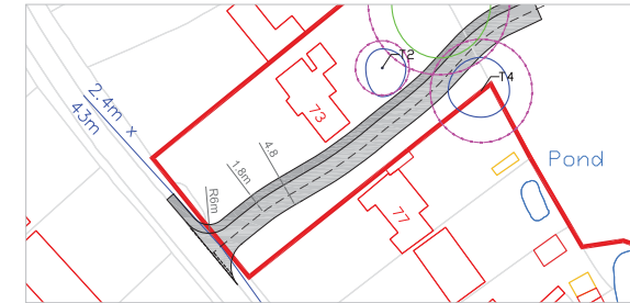
Indicative proposed site access. A 'no-dig' solution would be employed where the road passes between existing trees.
